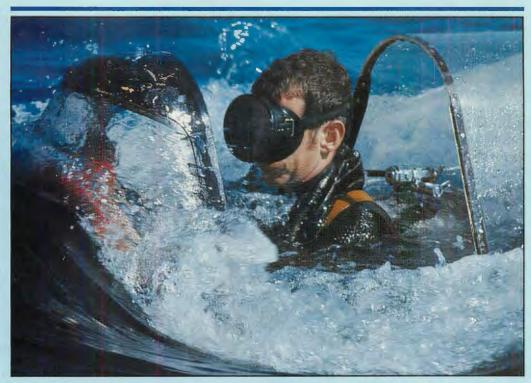
A member of UDT-21 surfaces in 1973 off Puerto Rico in an SDV (a Convair-14). SDV's 24-volt motor was powered by a series of batteries, good for several hours. Underwater, the SDV had a speed of about 4 knots. It could carry four men with individual SCUBA gear; during movement, they used "boat air" from eight SCUBA tanks mounted inside. Vehicle's two ballast tanks, amidships, enabled driver to attain neutral buoyancy and ascend or descend.
